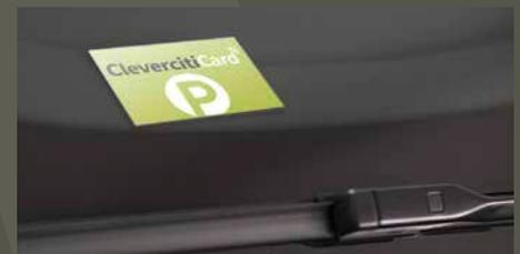
Leverage the ClevercitiCard as a digital permit, allowing for access control and precise space availability data in indoor or outdoor environments with limited infrastructure investment. The card sits in the vehicle's windshield and gives the parking operator exact position, occupancy, and identification data.
